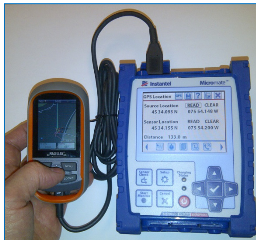
GPS Connected to Micromate
