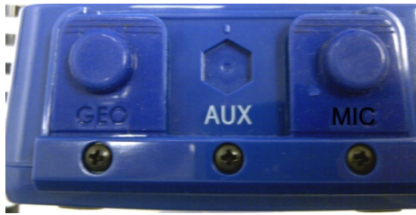
Protective Dust Caps without Optional AUX Connector
