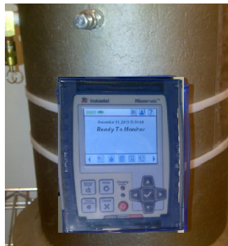
Micromate Attached with Plastic Tie-wraps
