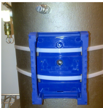
Micromate Attached with Plastic Tie-wraps
