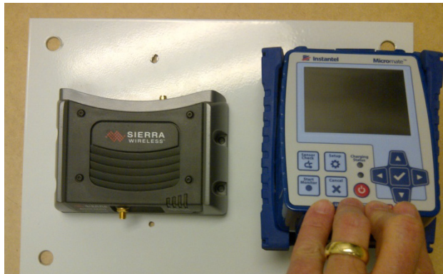
Install the Micromate in the Protective Boot
