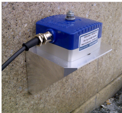
Geophone with Wall Mount Bracket
