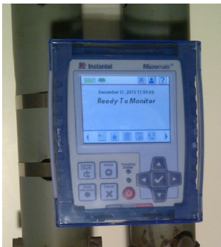
Micromate Attached with Metal Straps
