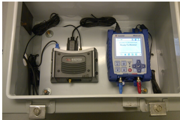
Mounting Panel Installed in the Enclosure
