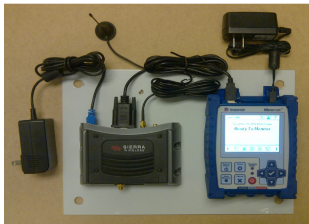
Placement of Modem, Micromate and Cables
