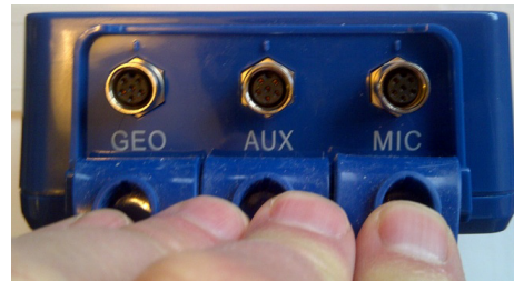
Dust Caps Pulled Back to Access Connectors
