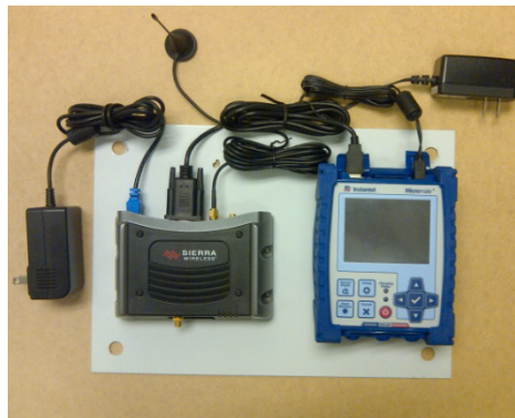
Micromate Connected to Modem
