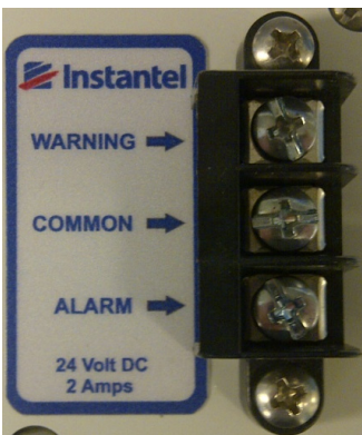
Remote Alarm Terminals
