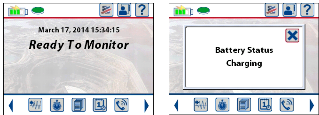
Micromate with External Power Connected Result of Touching Battery Icon
