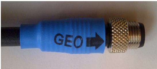
Geophone Cable Connector
