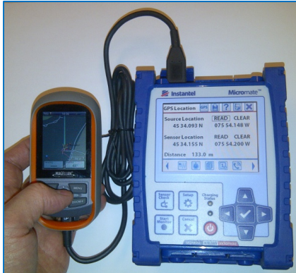
GPS Connected to the Micromate
