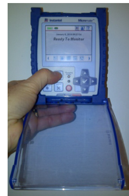
Wall Mount (cover opens down)
