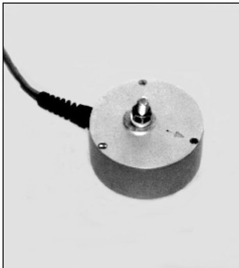
Figure 3-6 Bolting the Standard Transducer to a Surface.
