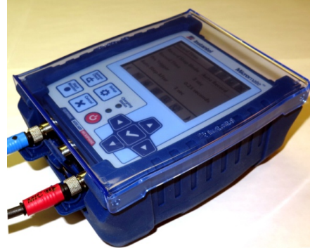
Micromate Installed in the Protective Boot
