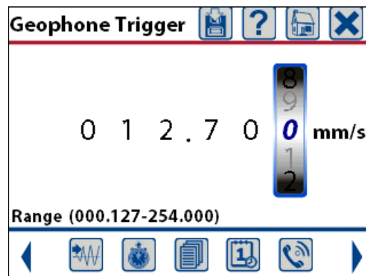
Geophone Trigger Level Set to 12.7 mm/s
