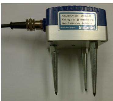
Geophone - Spikes Installed
