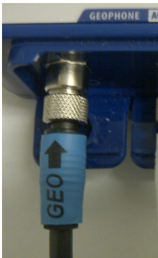
Geophone Connected to the Micromate
