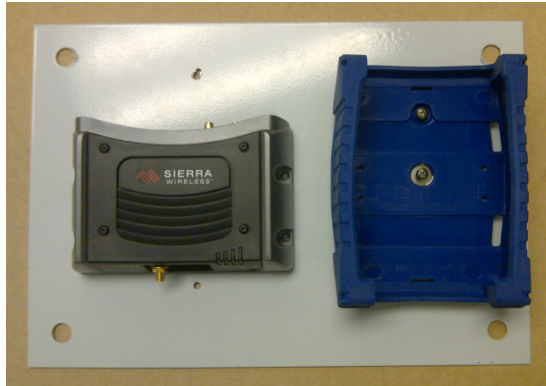
Modem and Protective Boot Secured
