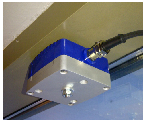
Geophone Mounted to the Ceiling
