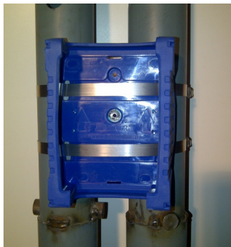
Micromate Attached with Metal Straps
