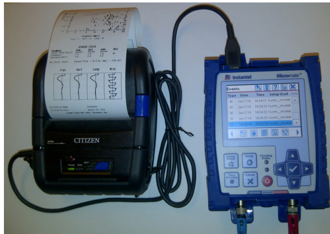
Micromate Connected to Citizen Printer
