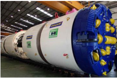
3.7 m (12 ft) Diameter Tunnel Boring Machine
