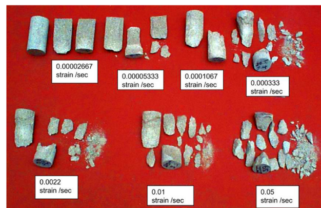
Higher strain rates promote fragmentation, collected samples after blasts.
