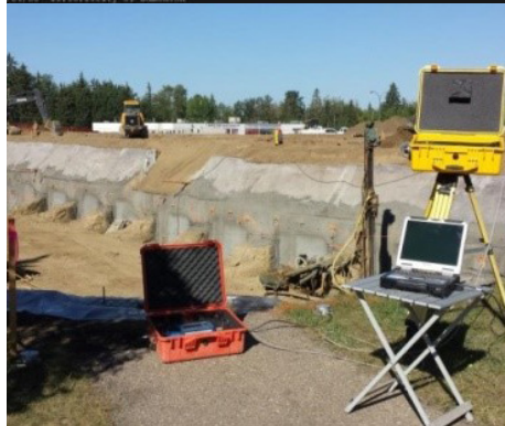
TOP PHOTO: INSTANTANEOUS PHOTO CAPTURE OF A TRIGGER VIBRATION EVENT. BOTTOM PHOTO: MONITORING VIBRATION LEVELS AT A CONSTRUCTION SITE WITH PHOTO CAPTURE.
