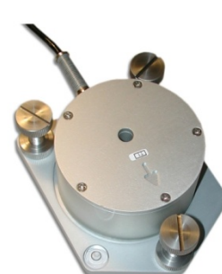
Figure 10 Bolting the Standard Transducer to a surface using the Leveling Plate.
