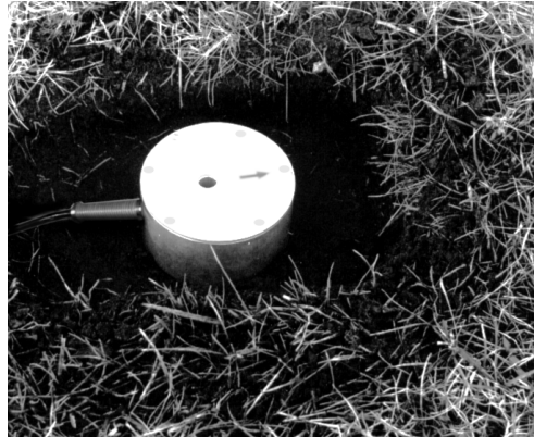
Figure 7 Burying the Standard Transducer.
