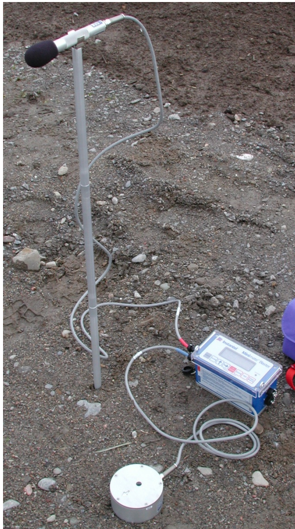
Figure 1 Installing the Minimate Blaster.
