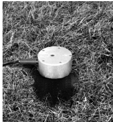
Figure 6 Final Installation with Ground Spikes Pushed Fully into the Ground.
