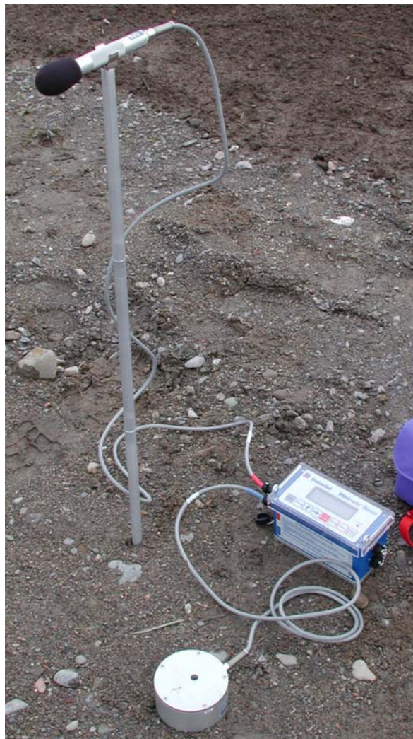
Figure 1 Installing the Minimate Blaster.
