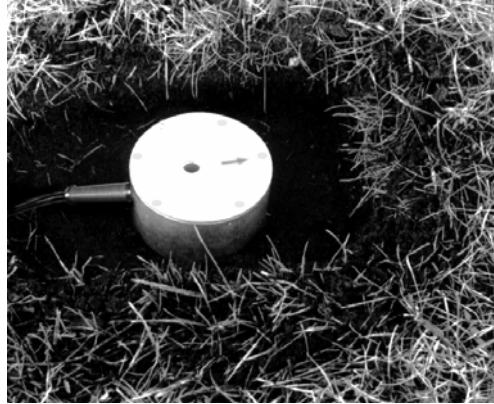
Figure 7 Burying the Standard Transducer.
