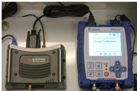
The Micromate units are tested and fully compatible with **Sierra RV-50, LS-300, and GX-400** modems. Example of the GX-400 modem, using the AirLink Ace Manager software to configure the modem.
