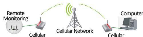
**NOTE** The Auto Call Home feature and connecting to a unit (to configure the unit from THOR) using remote communications requires a cellular modem. InstanTEL recommends using the Sierra Wireless™ AirLink™ GX-400, LS-300 series or Raven RV-50 modems.
